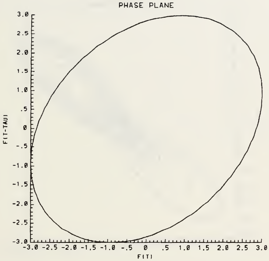
Figure 2.4 Pseudo-phase plane of a periodic signal.
